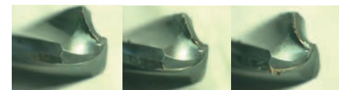
200穴 1000穴 2000穴 200 holes processing 1000 holes processing 2000 holes processing
